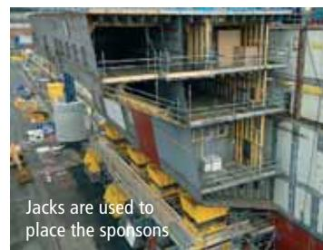
sections of the flight deck, it's crucial they are aligned with absolute precision while they are integrated into the build.
